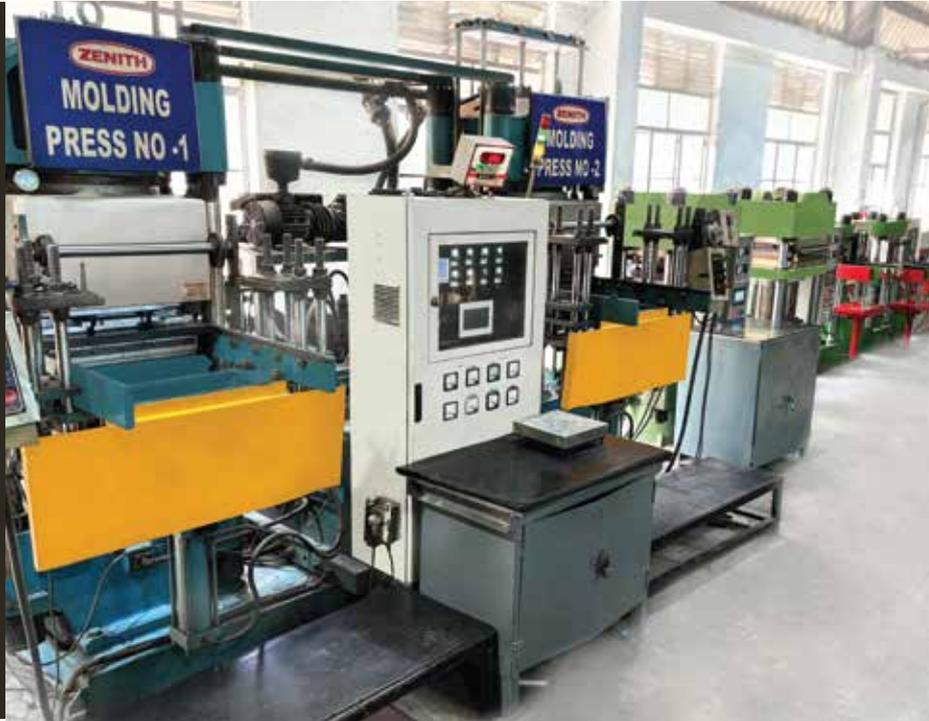
Zenith Manufactures wide range of custom rubber molded products in polymers like EPDM, NBR, CHLOROPRENE, SILICONE, FLURO SILICON, FKM, ACM, AEM (VAMAC) , SBR, NATURAL RUBBER. We produce molded products by using compression molding, transfer-molding process. Special controlled processes are developed by Zenith to produce such high performance molding products.
